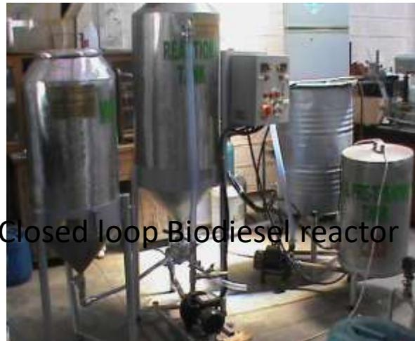
Closed loop Biodiesel reactor
